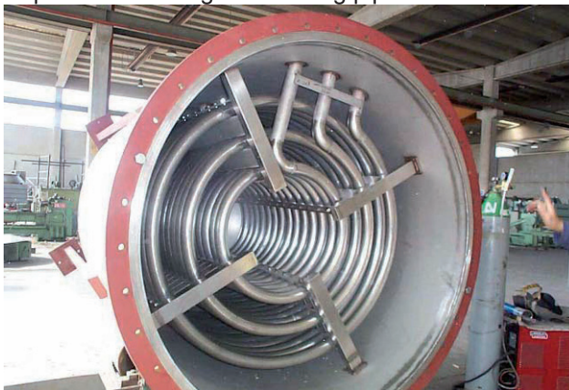
Serpentine / Cooling and heating pipes
